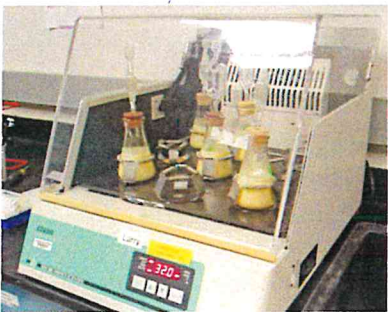
(Top Image) Overall view of the pilot plant at NCERC. (Bottom Image) The shaker flask systems for corn ethanol research at NCERC.
